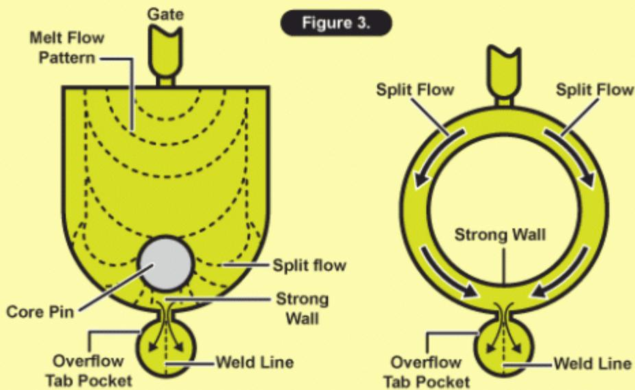
Improved weld line by using overflow tab pocket. Taken from *The Complete Part Design Handbook*
