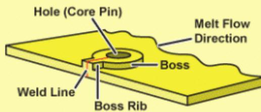
Improve boss strength using a rib on weld line location.
