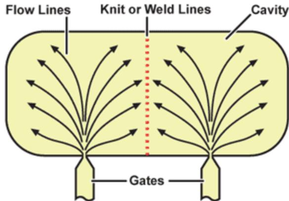
Knit line in a multi-injection-point cavity.
