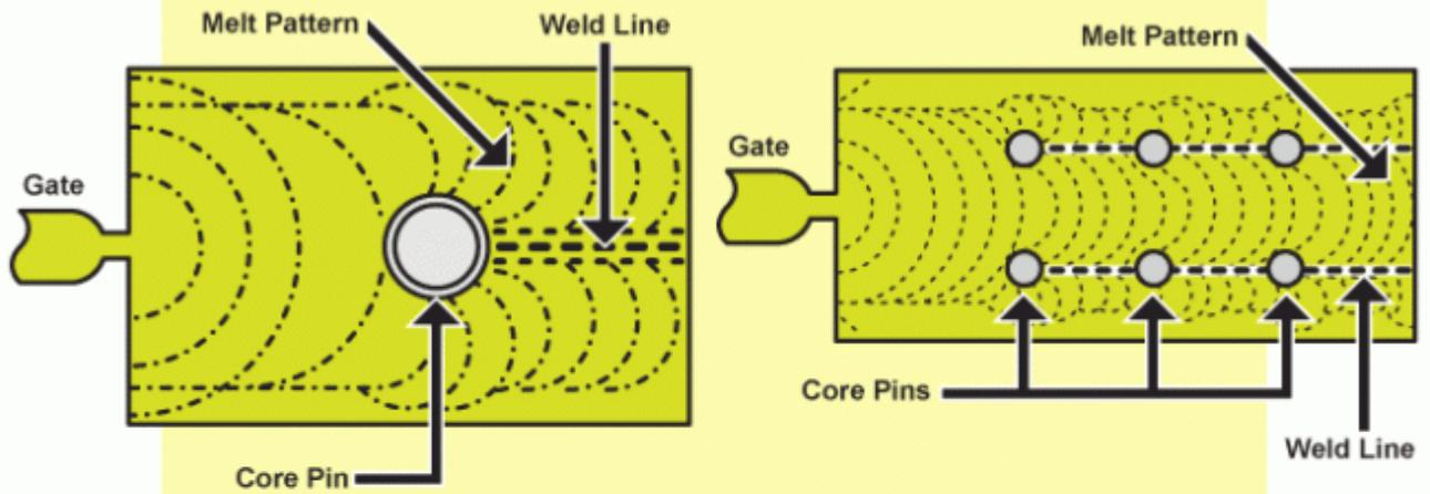
Weld line forms when melt flow splits around core pins.
